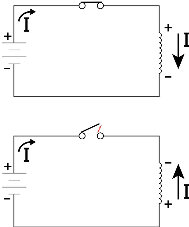
This returned high voltage spike can cause arcing of relay contacts as the high voltage looks for a path to dissipate, greatly shortening relay life. The negative voltage can also travel to other sensitive devices in the system, causing problems such as lockup of microprocessors, false triggering of overcurrent protection, and possibly damaging devices within the system.
