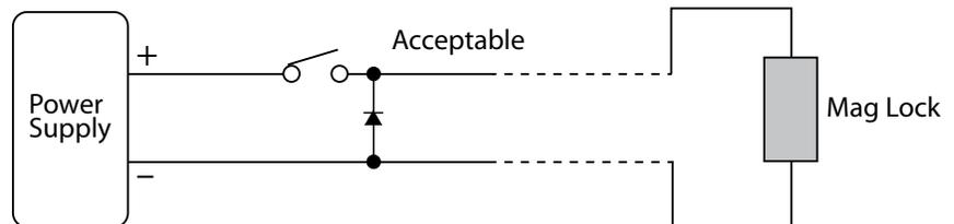
When using an external diode, most any general purpose power diode will work. Avoid small signal diodes, as they cannot handle the voltage and current levels generated by the back-EMF of most locks. The 1N4000 series is inexpensive and easily obtainable and works well as back-EMF protection.
