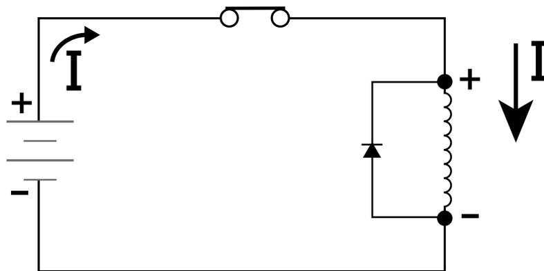
When the switch is opened, the negative voltage will flow back through the diode, returning to the lock to be dissipated by the lock's internal resistance.
