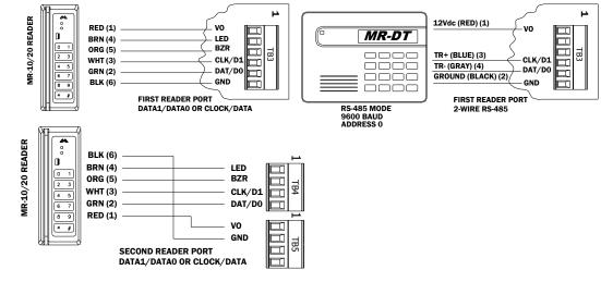
When powering any remote device(s) by the MR51e, care must be taken not to exceed the maximum current available. Cable gauge must also be evaluated. See specifications section for details.
