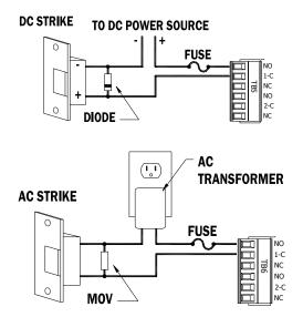
Diode Selection: Diode current rating: 1x strike count Diode breakdown voltage: 4x strike voltage For 12 Vdc or 24 Vdc strike, diode 1N4002 (100V/1A) typical.
